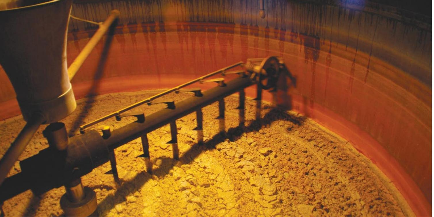
(ABOVE) Kettle used in the first stage of brewing, called lautering and sparging, is stirred to assist in draining off a liquid that is then boiled. (BELOW) Some of the miles of stainless steel pipe running through the new brewery. (BOTTOM) Fermentation tanks where yeast is added to wort, the liquid produced by boiling. The yeast converts sugars in the wort to ethyl alcohol and carbon dioxide gas. The result is beer.
